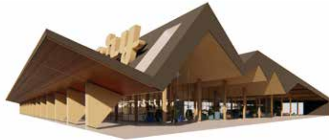
Above, a folding CLT ceiling at this big box grocery shapes space and integrates cooling and heating systems, lighting, plumbing, electrical systems, and skylights. Below, the folding roof cantilevers to create urban wood rooms: an entry porch, a dining porch, and a fulfillment zone on the other side.
