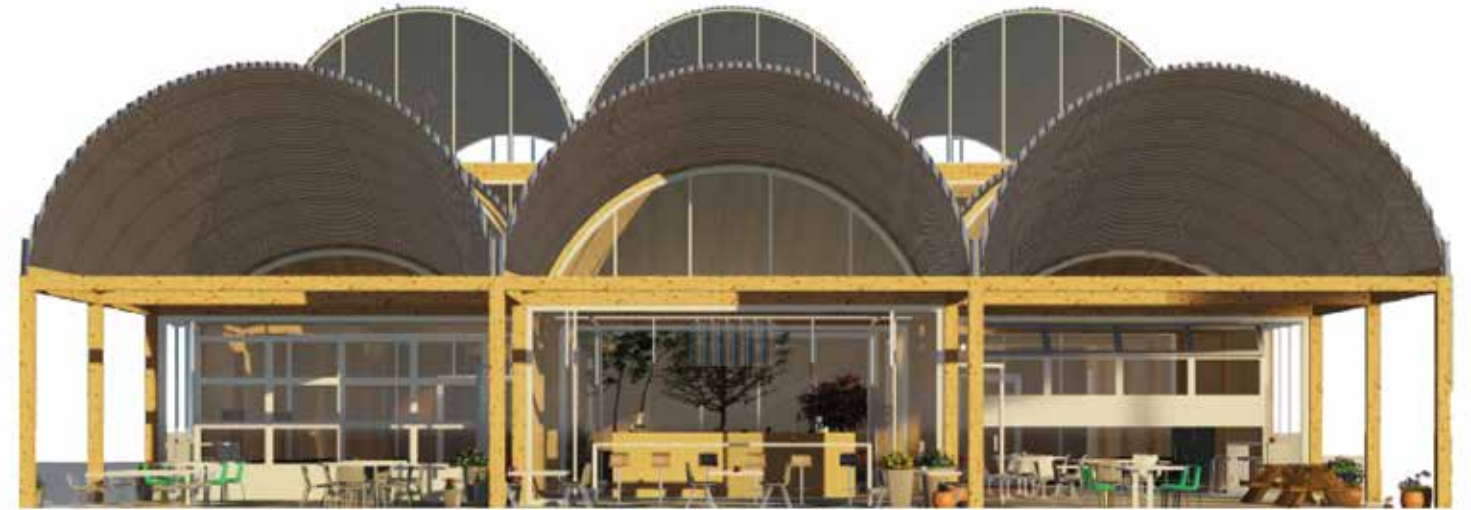
Above and bottom, barrel vaulted metal arches sit atop glulam frames for the visitor pavilion and production shed of a metal warehouse that houses a roastery.
