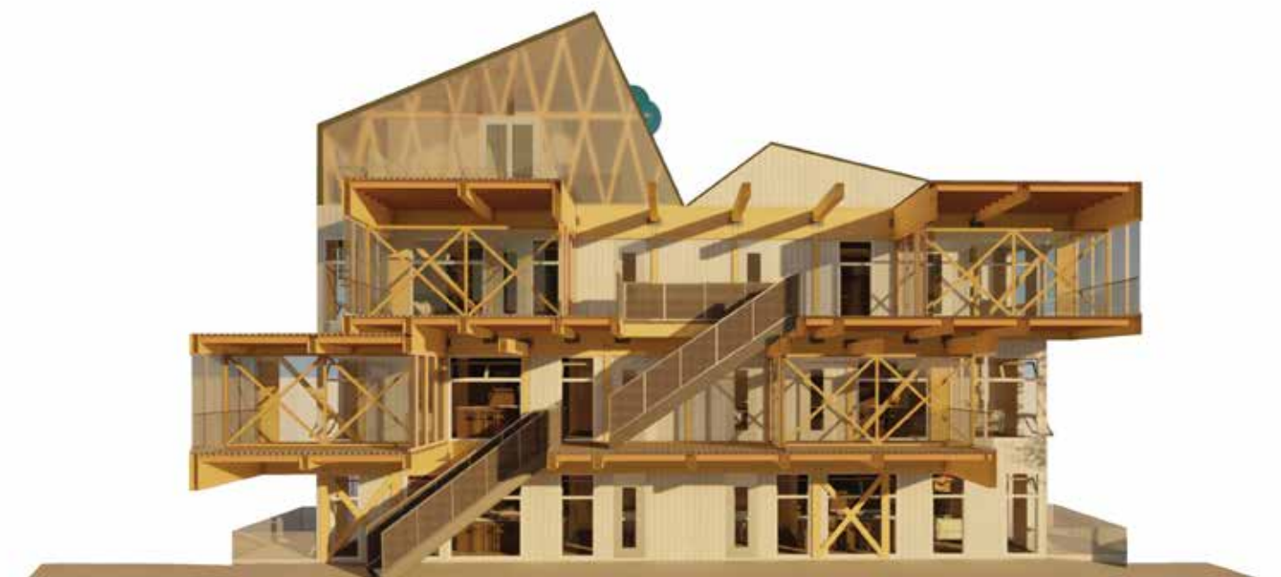
Stacked glulam trusses — made from rectangular rather than triangular frames — extend the living space of these garden apartment units through patios, screened porches or rooftop decks.
