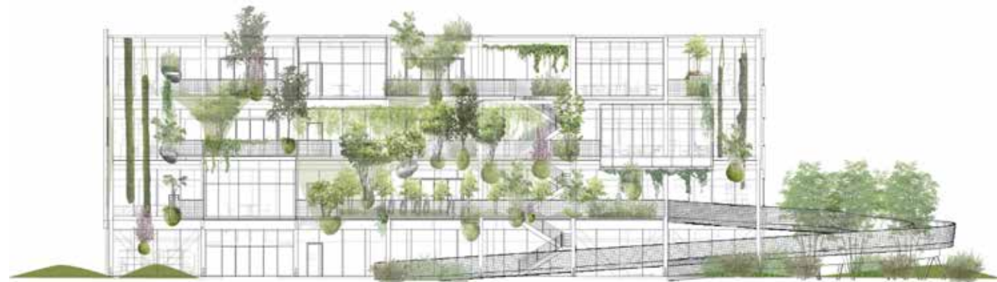
Above, access to outdoor terraces at this tenant office improves working conditions and indoor air quality. Below, a thickened façade hosts vegetated terraces, meeting rooms, a bike ramp and the front entrance.
