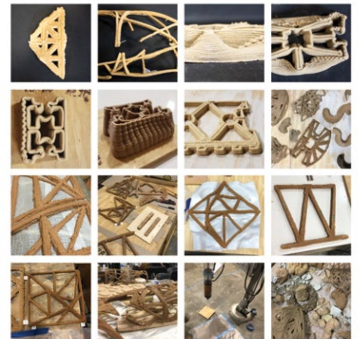
Numerous printing experiments were done to refine the wood paste mixture and printing process.
