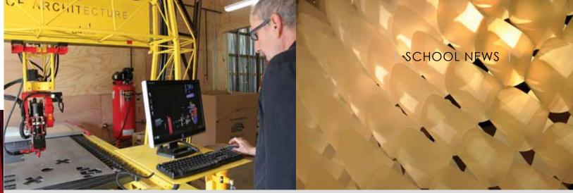
Santiago R. Perez operates the computer on this custom-made machine that does computer numerically controlled plasma cutting and five-axis milling.
